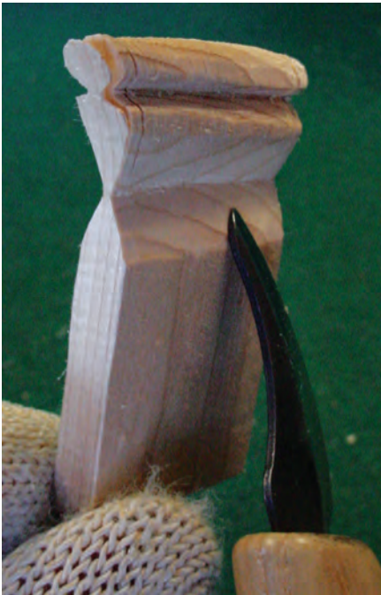
10. After all the feathers are rived, trim off the lower side of the hinge. Make it a flat plane.
