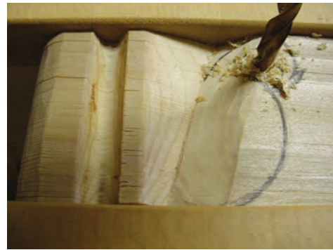
22. Drill a hole in the space between the curved-neck and the breast.
