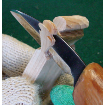
9. Rive the feathers, starting at the head side. Because of the small size, a single-handed Flexcut™ riving knife works well.
