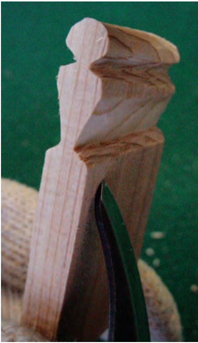
8. Carve the hinge ...1/3 on each side ...leaving 1/3 for the center.
