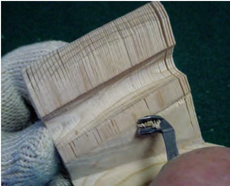
30. Make a v-cut with a Flexcut™ 70-degree v-scorp just under the buffer zone. Once fanned out, the decorative detail will be revealed.
