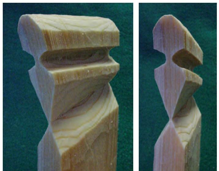
20. Trim the lower part of the short taper. Make a nice flat plane. This area needs to be open so the feathers can turn freely and interlock without butting up against the bird's body. Do this on both sides of the blank.
