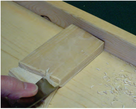
17. Trim the hinge to make it more narrow. It should now be about 1/16-inch. The extra width was necessary during the slicing process to maintain structural integrity while riving.
