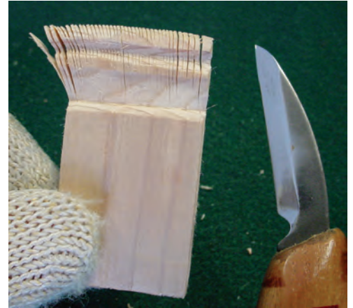
9. Rive the feathers, starting at the head side. Because of the small size, a single-handed Flexcut™ riving knife works well.
