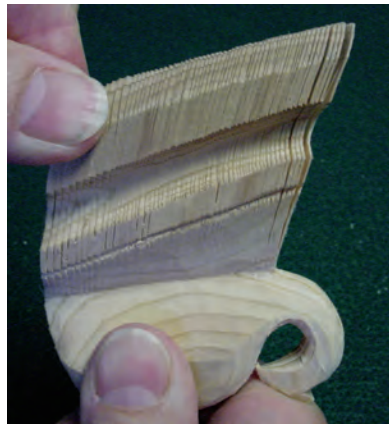
31. Flex the feathers to loosen the fibers at the hinge so they will turn more easily when interlocking them.
