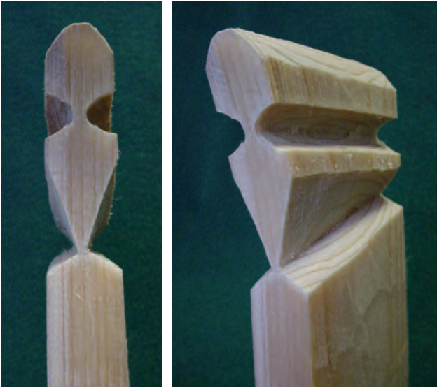
18. Check to insure an even amount of wood was removed from each side and the base of the hinge is centered. It is at the base that the feather will pivot to be interlocked.
