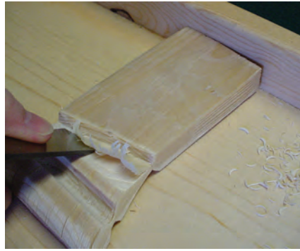
17. Trim the hinge to make it more narrow. It should now be about 1/16-inch. The extra width was necessary during the slicing process to maintain structural integrity while riving.
