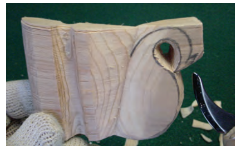
25. Shape the Pelican's body by removing the wood up to the top-knot of the Pelican's head.
