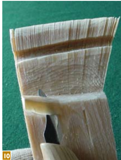
9-11 Photo 9: After the feathers are rived, use a knife or No.11 6mm gouge to trim the interlock and the hinge so they are narrower. They were left wider during the riving process so the wood would not wobble. The interlock centre should now be about 3mm (1/16in), the hinge about 1.5mm (1/16in). Photo 10: Next, trim the lower part of the short taper. This area needs to be airspace so the feathers can freely turn and interlock. Make a nice flat plane. Photo 11: Next, draw the dove onto the blank
