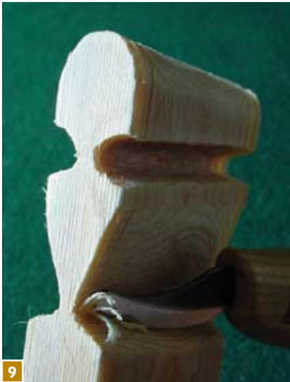
9-11 Photo 9: After the feathers are rived, use a knife or No.11 6mm gouge to trim the interlock and the hinge so they are narrower. They were left wider during the riving process so the wood would not wobble. The interlock centre should now be about 3mm (1/16in), the hinge about 1.5mm (1/16in). Photo 10: Next, trim the lower part of the short taper. This area needs to be airspace so the feathers can freely turn and interlock. Make a nice flat plane. Photo 11: Next, draw the dove onto the blank
