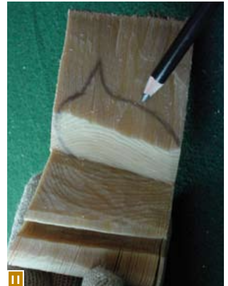
9-11 Photo 9: After the feathers are rived, use a knife or No.11 6mm gouge to trim the interlock and the hinge so they are narrower. They were left wider during the riving process so the wood would not wobble. The interlock centre should now be about 3mm (1/16in), the hinge about 1.5mm (1/16in). Photo 10: Next, trim the lower part of the short taper. This area needs to be airspace so the feathers can freely turn and interlock. Make a nice flat plane. Photo 11: Next, draw the dove onto the blank
